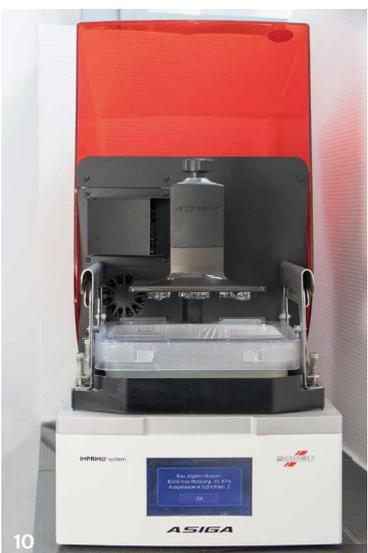
**Fig. 9:** It is also possible to enter the measurements in a table and specify the limit values. **Fig. 10:** The DLP 3D printer Asiga MAX™.
