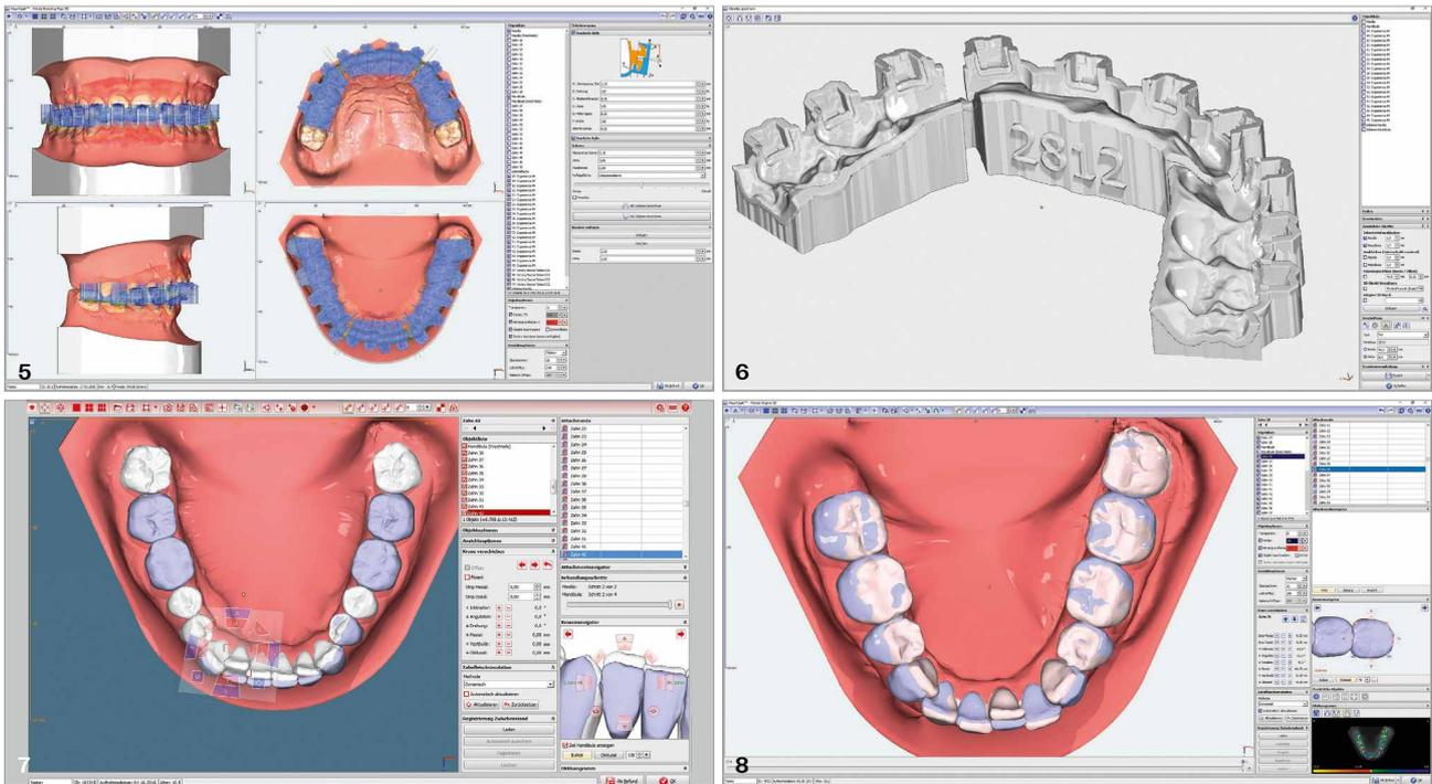
**Fig. 5:** The tray is calculated and saved. **Fig. 6:** The tray can be labelled with a unique number and exported as an STL file. **Fig. 7:** The customised target setup is generated in the Aligner 3D module. **Fig. 8:** The extent of the planned tooth movement can be visualised by superimposing the final finding over the initial finding.
