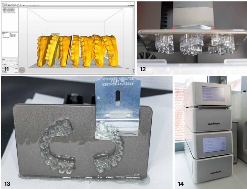
**Fig. 11:** Arrangement of the IDB trays in the Asiga Composer software. **Fig. 12:** The printed trays suspended from the build platform of the Asiga MAX™. **Fig. 13:** A glass scraper or similar tool can be used to detach the trays and printed models from the build platform. **Fig. 14:** The cleaning and light-curing device from rapidshape.
